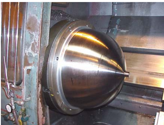
Figure 10: A Machined Hemispherical Head
