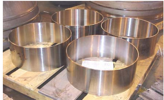
Figure 11: Machined Cylindrical Center Sections.
