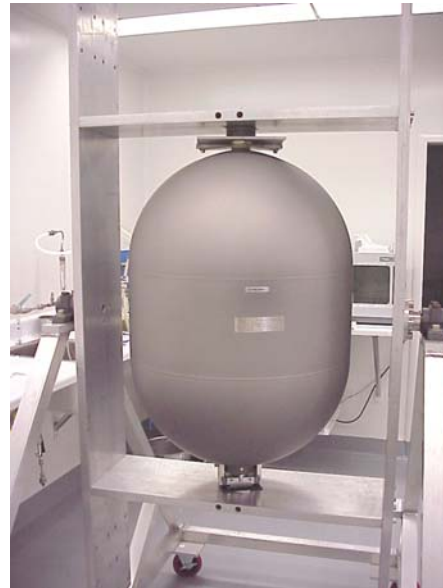
Figure 14: A Completed Tank at Final Clean
