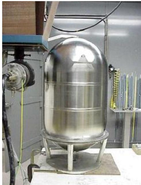
After closure the tank assembly is stress relieved in a vacuum furnace to remove residual stress from the weld operations. See Figure 21.
