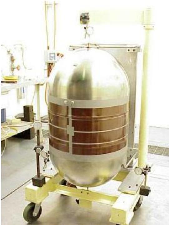
**Pressure Cycles Tests:** The propellant tank was cycle tested with a total of 16 proof and 100 MEOP pressure cycles. Pressure testing was conducted hydrostatically. Both proof and MEOP test pressures were temperature adjusted to test the worst case conditions.
