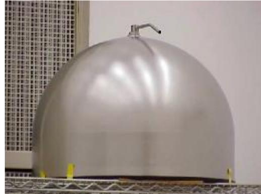
The mounting hemisphere was also eb welded to a cylinder extension, solution treated and aged, and finish machined. However, part of the finish machine process also included eb welding three tabs to the mounting hemisphere and final machine these mounting tabs. A finish machined mounting hemisphere is shown below in Figure 16.
