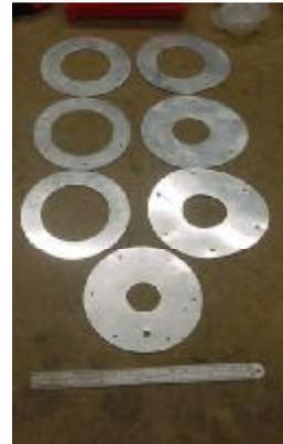
The data collected from the drop tower test supported a tank design with two annular ring baffles. The baffles are located on the tank cylindrical section approximately 8 inches apart and equal distance from the tank mid-plane. Both baffles are identical in size - approximately 8 inches wide with a 7-inch "hole" in the center of the baffle.
