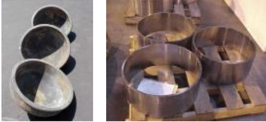
The outlet hemisphere and its cylinder extension forgings were rough machined and electron beam (eb) welded together, as shown in Figure 14.
