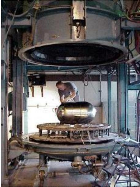
Following closure weld, a boomerang was installed to the propellant hemisphere as shown in Figure 22. The boomerang is used for strut connection.
