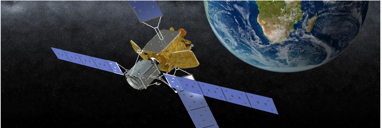
Space Logistics LLC, a wholly owned subsidiary of Orbital ATK, provides cooperative in-orbit satellite life extension and maneuvering services to geosynchronous satellite operators using its Mission Extension Vehicle (MEV). The MEV docks with customers' existing satellites providing the propulsion and attitude control needed to extend their lives.
